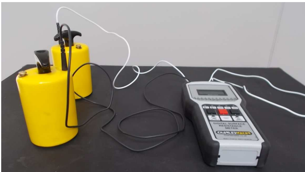
Fig.1: The equipment and the two measuring electrodes used for the tests
